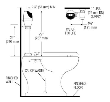
The Model 8115 valve is designed for installations where the water supply is roughed-in 24" (610 mm) above the top of the water closet.
